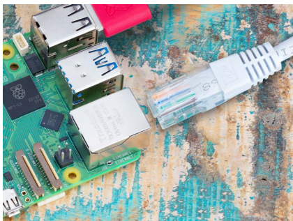
Figure 2-17 Connexion Ethernet du Raspberry Pi 5
