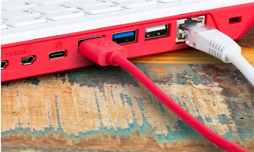
Figure 2-23 Connexion Ethernet du Raspberry Pi 400
