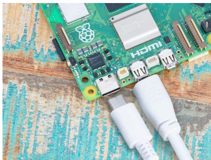
Figure 2-18 Alimentation du Raspberry Pi 5
