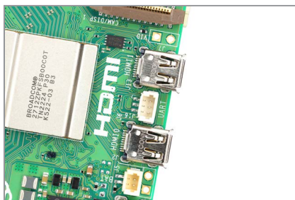
Figure 1-12 Ports micro HDMI d'un Raspberry Pi
