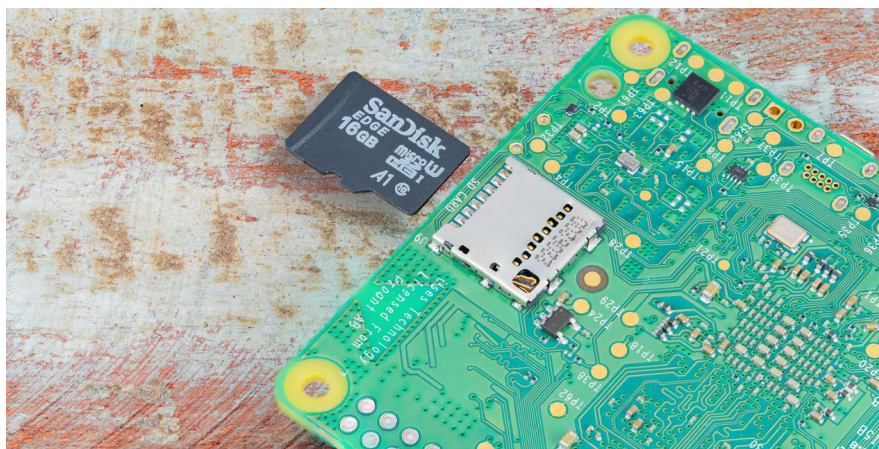
Figure 2-13 Insertion de la carte microSD
